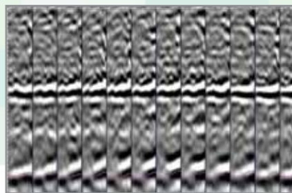
Automatic RMO picking along 12 azimuthal sectors extracted from 3D reflection angle gather
